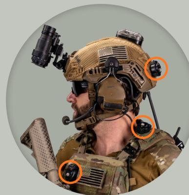
If you are wearing the gauges, they are designed to be attached on the head (e.g. back of the helmet), non-firing shoulder, and chest. The gauges are color coded with letters on the back: H for Head (Orange), S for Shoulder (Gray), C for Chest (Blue).
