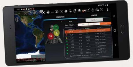
**Mobile Connectivity:** The Blast Gauge System App (BGSA) for AndroidTM and the Android Team Awareness Kit (ATAK) allows for near real-time data analysis and download with Bluetooth 4.1.
